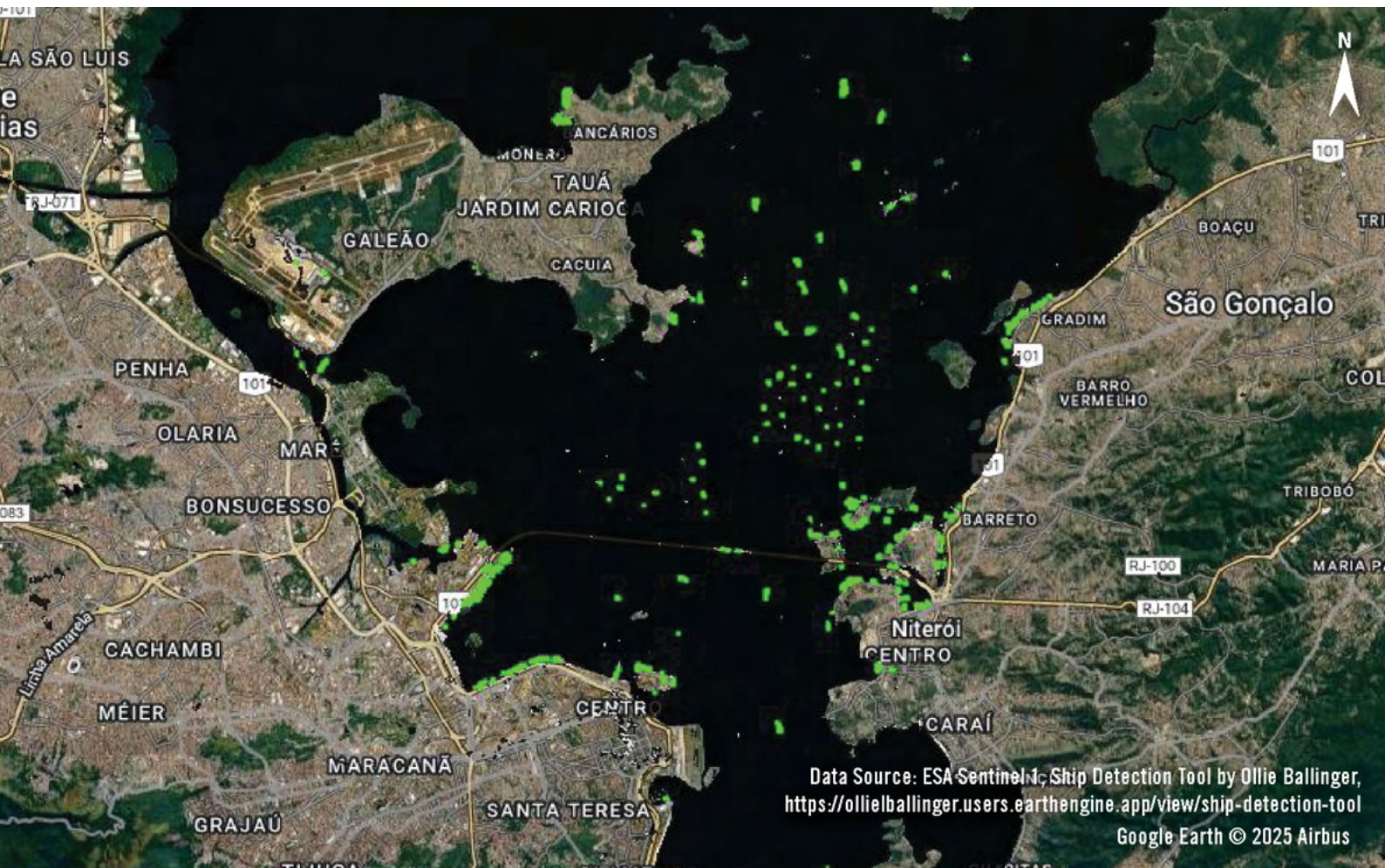
Map showing the results from the SAR detection tool from 20 February 2025. Ships detected with the tool are highlighted in green. Ships are visible throughout the bay, including heavy concentrations along the coast of São Gonçalo., Rio de Janeiro (Brazil).
