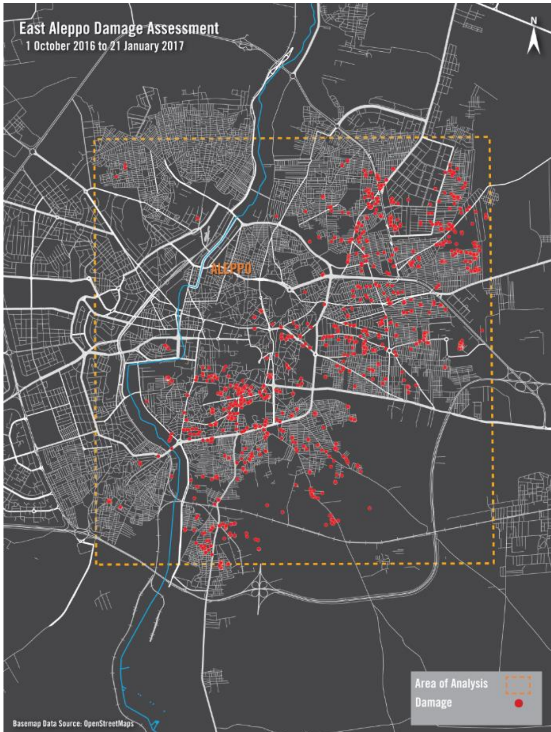
Satellite imagery analysis comparing data from 1 October 2016 and 21 January 2017, and showing structures in an area of eastern Aleppo city of 65km 2 that were damaged or destroyed during that period.
