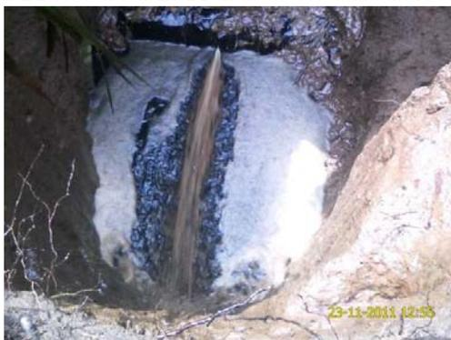
the photograph the oil is seen to be still flowing. Accufacts noted that the reported volume of 6.8 barrels was “unlikely, given spray pattern shown on 6 inch pipe.”<sup>85</sup>
