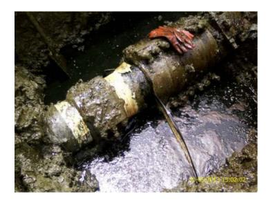
In another case, a spill occurred at Ikarama in Bayelsa state on 24 May 2013. The JIV, which took place on 30 May, six days later, found the spill was due to a hacksaw cut. 64 However, the photograph (reproduced above, taken from Shell's website) does not show a hacksaw cut. According to Accufacts: "Most likely this photo suggests that the seal on a previous clamp repair has failed for various reasons, such as poor installation." 65
